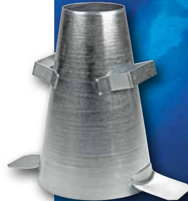
ASTM C1611/1611M – Slump Flow
